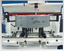
Cylinder Heads with long studs can be set up without having to remove the studs.
