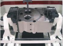
Fixturing and Tooling to handle repair processes such as Valve Seat Machining, Seat Ring Replacement, Valve Guide Reaming, Injector Tube Repairs, etc.
